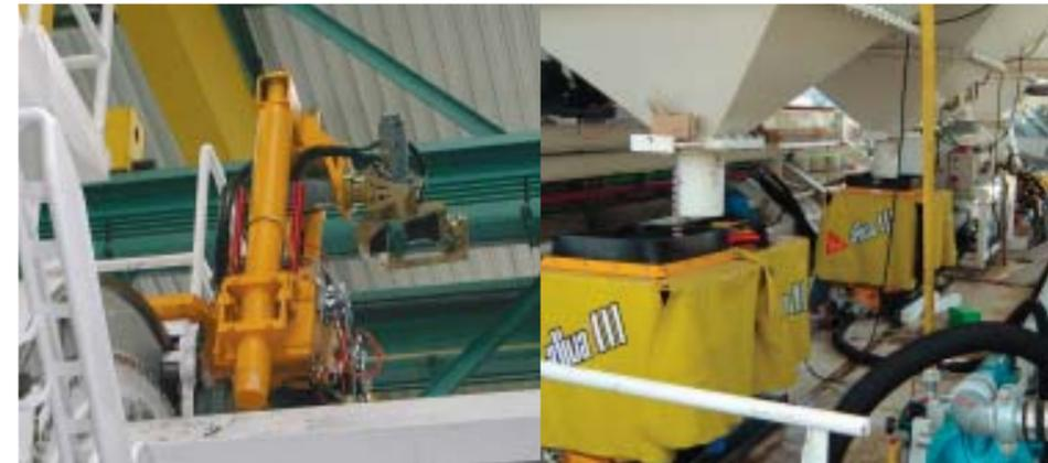
Temporary spraying robot with 800 mm telescoping range, mounted on the live ring of a drilling mount
