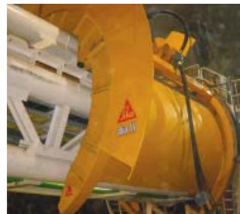
Spraying robot in the L2 zone
