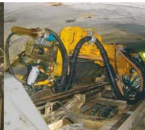
Spraying robot with three-stage spraying boom
