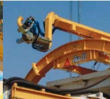
Spraying robot with one-stage spraying boom
