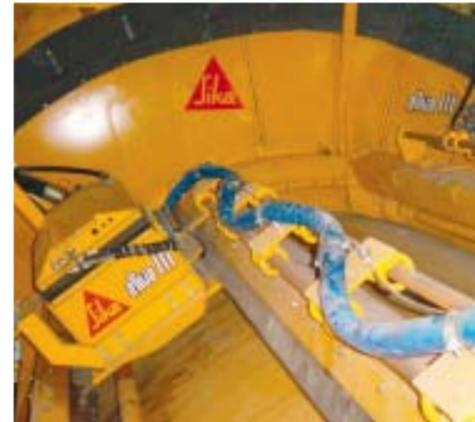
Spraying robot with two transverse moving gears
